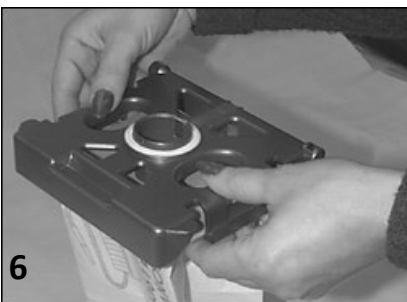
Fig. 6 Ensure the new Filter Bag is securely fitted under the tabs on the Retainer.
