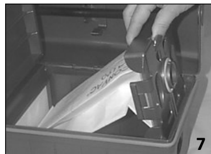
Fig. 7 Refit the Retainer with Filter Bag attached
